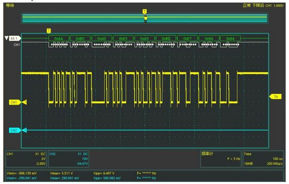
10. If the length of the acquired waveform is not enough, the fixed sampling rate can be reduced, but it is necessary to ensure that the baud rate of the measured signal is more than 10 times when the sampling rate is taken.
